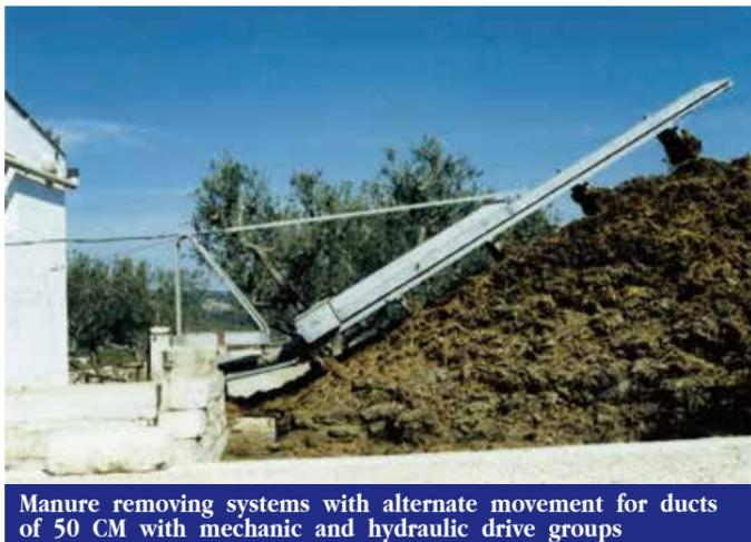
Manure removing systems with alternate movement for ducts of 50 CM with mechanic and hydraulic drive groups
